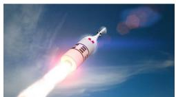
They recently carried out a successful test of a Launch-Abort System (LAS) for the Orion capsule designed to take U.S. astronauts to the Moon. It is designed to activate in the event of a rocket malfunction, on the pad or in flight. The LAS consists of three different types of solid-fuel rocket
